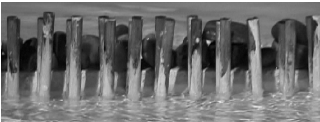
Figure 8 – Physical model of north jetty deck improvement with second row of pilings.
